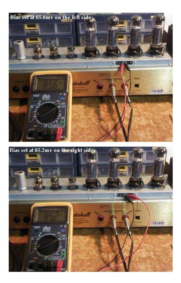
It worked!!! For the next 5 hours I kept on monitoring the Bias voltage and it was steady as desired!
