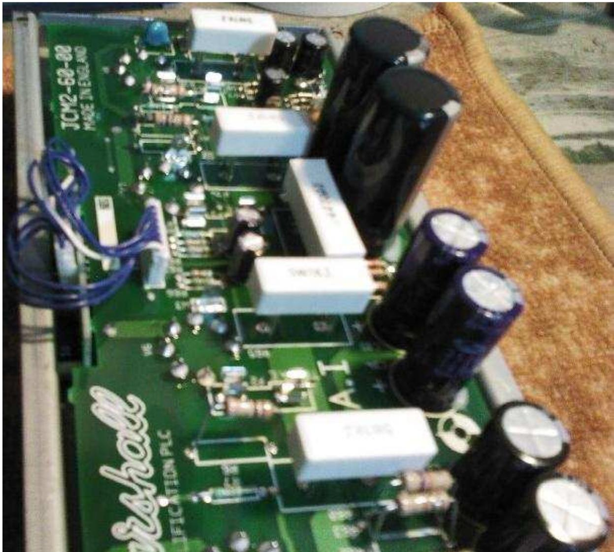
Right after this I plugged in the amp to an A.C. voltage limiter allowing a few seconds for the new caps to fill up slowly. Turned up the voltage to 120v, waited a few minutes and checked the Bias. It held steady for about an hour now, but then it'd start to drift like it did before. I felt really disappointed
